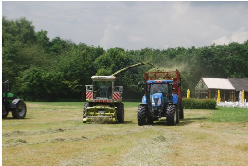
*3. Forage harvester, picking up and blowing grass into the wagon*
