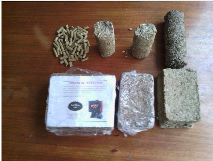
*Picture 1: Final products - pellets and briquettes*
